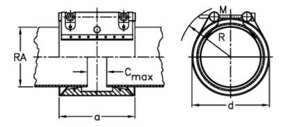
a = 77.4C max with insertion band = 17d = 85M (screw) = M8Nominal pressure (bar) = 16R = 105RA = 63.0RA min-RA max plastic = 62,5-63,5
